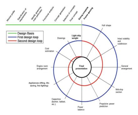
Fig. 1 Ship design spiral, adapted from Evan's ship design spiral (Evans 1959) by Linda de Vries and Per Hogström at Chalmers Technical University. Used with permission
